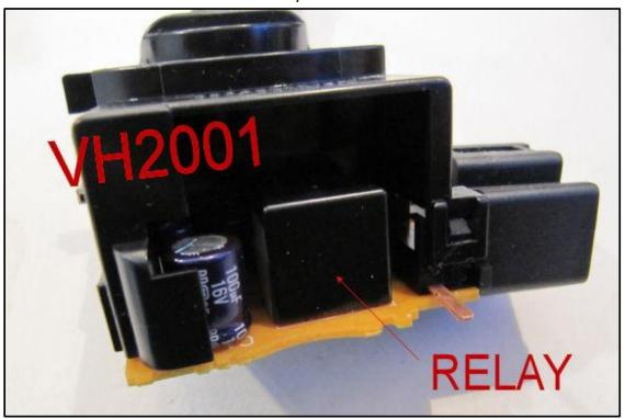
STEP #3: Locate the solder points for the bad relay...
